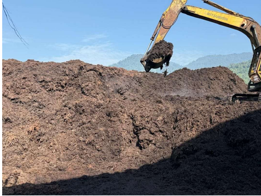
Figure 2. The EFB dump being worked. Fresh and partially decomposed empty fruit bunch is consolidated by a tracked excavator into the standing mass of the disposal site. The darkened, matted material in the foreground is well into anaerobic decomposition.
