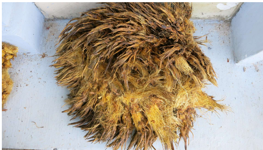
Figure 1. Prepared EFB fibre. The frondlets have been cut from the bunch and reduced to short lengths, at which point the individual fibres separate readily, giving the coir-like texture described in the text.
