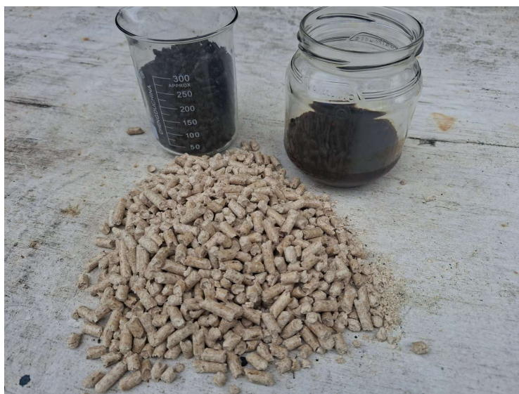
Figure 2. Inputs and products. Foreground: as-received softwood pellets. Left vessel: recovered biochar in a graduated beaker (used for bulk-density measurement). Right vessel: condensed wood vinegar.
